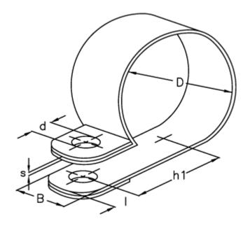
$\begin{array}{ll} d & = 6.4 \\ \text{Diameter D} = 20 \\ \text{h1} & = 19.7 \\ \text{I} & = 6.0 \\ \text{s} & = 0.8 \\ \text{Width B} & = 15 \\ \end{array}$
